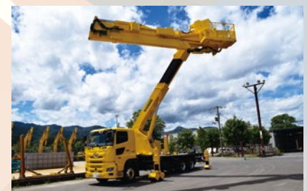
当社の橋梁点検車 Kanamoto Bridge Inspection Vehicle
